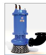
The "NSEW" Series is a unique designed submersible Slurry / Sewage pump comes with Non -Pressurize triple mechanical Seal Assembly to avoid hydraulic pressure of rotating part, So abrasive slurry does not affect the seal and motor
